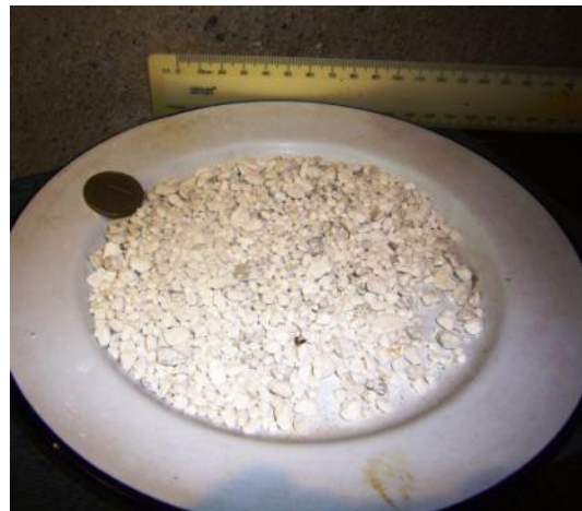
Dust reduced granulated quicklime for ease in handling and controlling. One Euro coin shown for grain size comparison.
