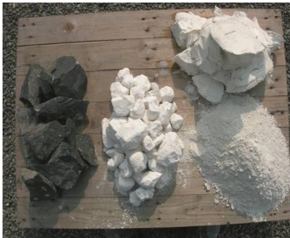
Transition of lime from limestone to hydrate with 'lumped' quicklime in the centre.
