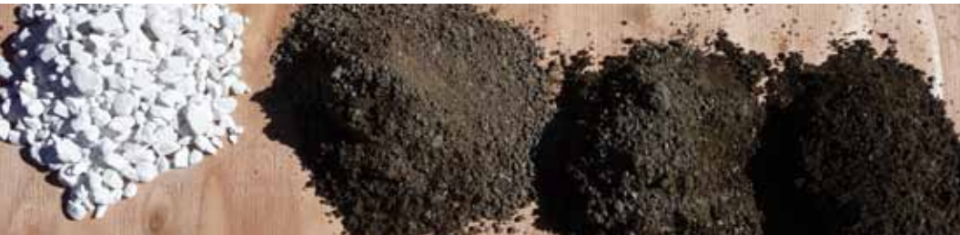
The basic materials for a hot mix lime mortar – quicklime and sand
