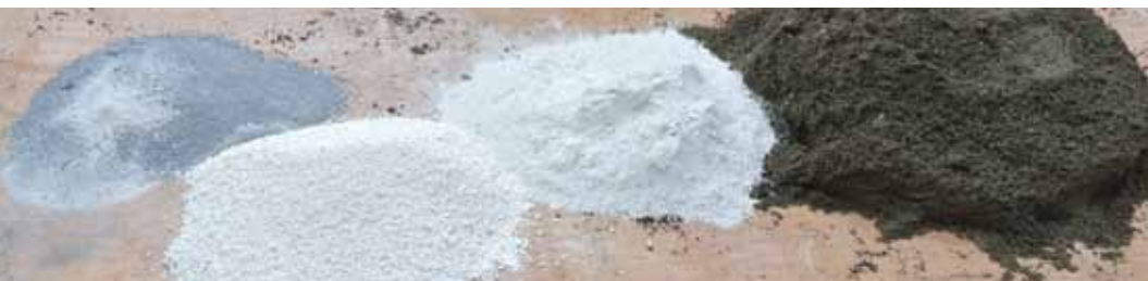
A more complex mix - natural hydraulic lime, quicklime, limestone dust and sand
