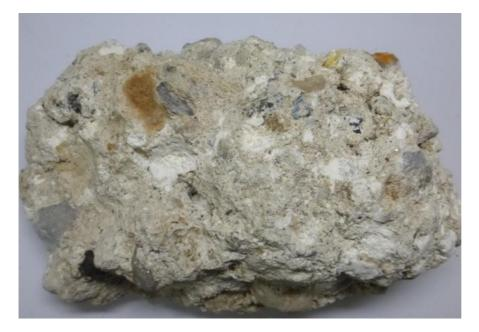
It is often quoted that if there are an abundance of inclusions within a mortar it is likely that it was mixed as a 'Hot-Lime' where the lime was added to the sand as a Quicklime and that it was used 'Hot'.
