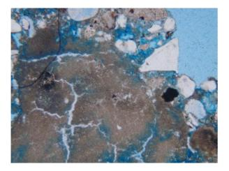
As with hot lime mixes variations in binder distribution throughout the mortar can be observed, and areas of dense
