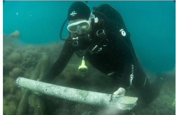
Chris Brandon of the ROMACONS project collects a sample of ancient Roman concrete drilled from a breakwater in Pozzuoli Bay, near Naples, Italy. The breakwater dates back to around 37 B.C. (D. Bartoli photo, courtesy of J.P. Oleson)
