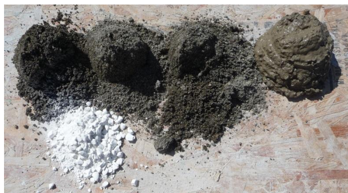
The mix decided on-showing 3 parts sand: 1 part clay and 6.7% quicklime
