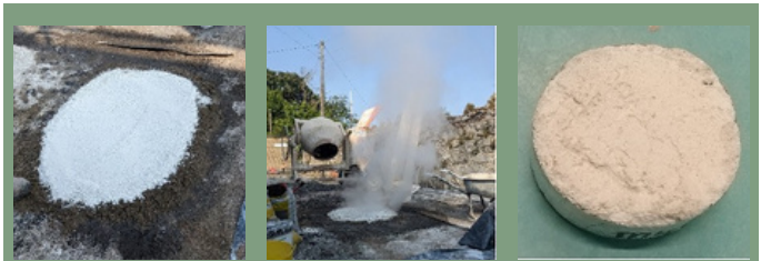
Fig 1. Preparation of quicklime samples (a) layers of quicklime and sand aggregate; (b) release of steam during exothermic reaction and (c) cylindrical samples
