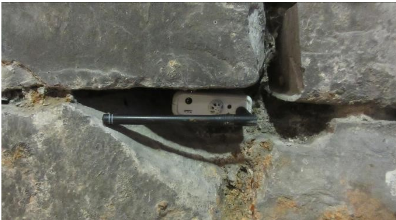
Monitoring of temperature and relative humidity at Dublin City Wall, Wood Quay Venue.
