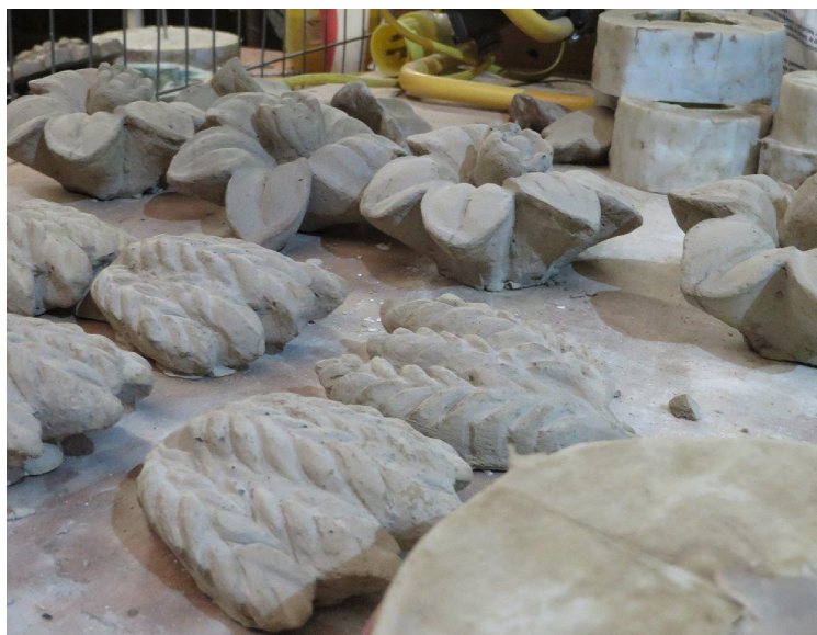
Left: Moulds for Roman cement casts. Above: Turned out Roman cement casts, drying before being prepared for fixing
