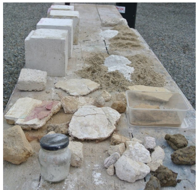
Materials including hot-lime mortar test cubes and aggregates
