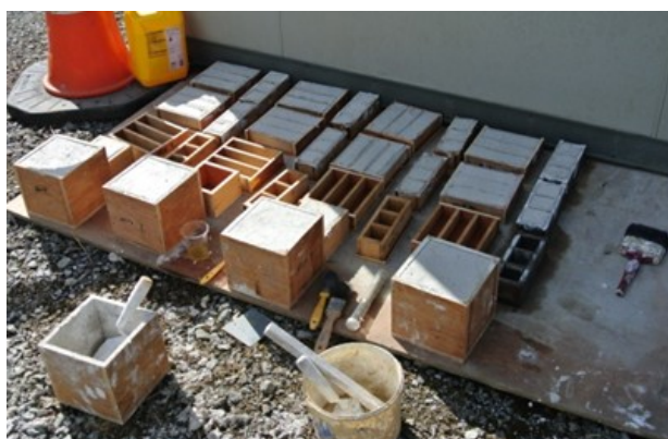
Hot-lime mortar test cubes
