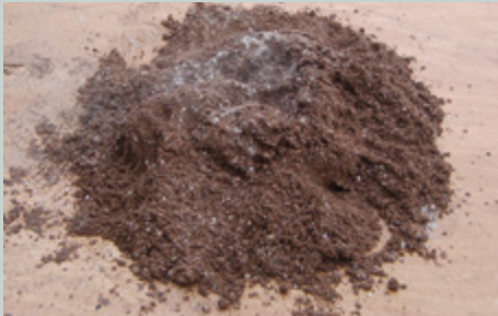
Fig. 9 Quicklime slaking with damp sand.
