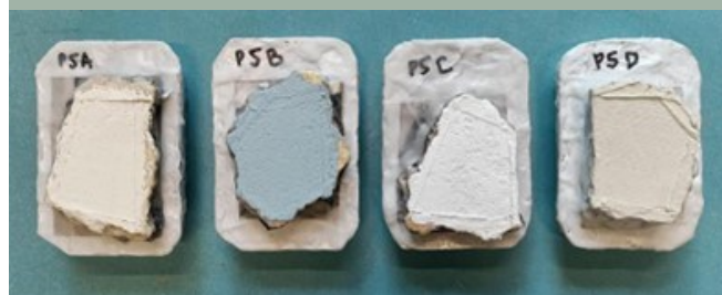
Painted lime plasters for vapour permeability testing.
